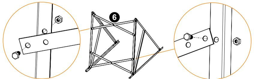
5. Screw the collector supporting part 5 to the bottom part of the frame and tighten the screws.
