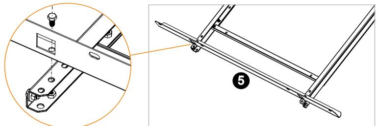
4. Screw the collector supporting part 5 to the top part of the frame without tightening the screws.
