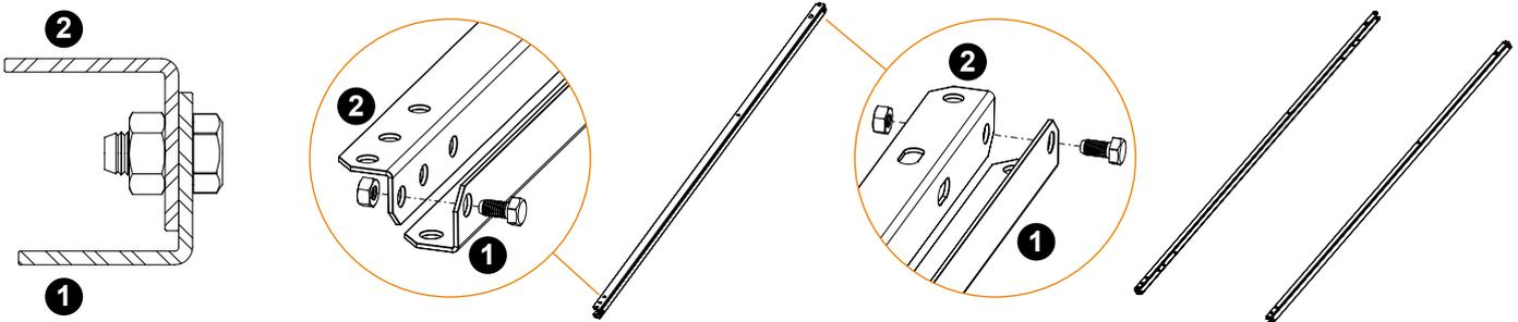
2. Place part 4 between the two  $\Pi$  shape parts constructed in the former step 1 in order for the frame to be formed. Screw straight parts 6 (which will be used for the mounting of the support base to the tiles) to the bottom part. Repeat for the rest of the parts.
