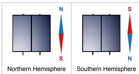
**Orientation - optimum angle:** a basic factor for the system's optimum performance is the selection of its angle and orientation for its particular location and the time during which the maximum gain is required. The solar system should be positioned so that the collector's surface faces the geographical south, if the installation takes place in the Northern Hemisphere (and the geographical north for the Southern Hemisphere), i.e. it should always face the Equator.
