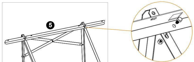
7. In case of two collectors, first place the left one at the bottom part **5**, lifting the upper part **5**. Place the screws and the collector's fixing washers (4 for each collector) without tightening them. Place mechanically tightened Ø22 unions at the edges of the collector.
