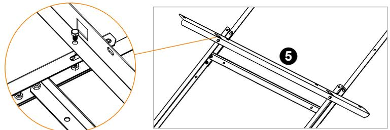
5. Bend the straight parts 6 of step 2 with the hand covering the beams of the tiled roof. Drill and fasten up with bolts. Use level so that the base is horizontally placed.
