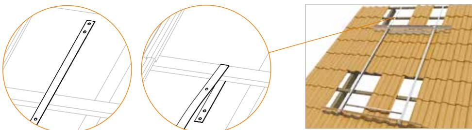
6. In case of two collectors, first place the left one at the bottom part 5, lifting the upper part 5. Place the screws and the collector's fixing washers (4 for each collector) without tightening them. Place mechanically tightened  $\text{Ø}22$  unions at the edges of the collector.
