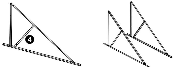
4. Place parts 6 crosswise and tighten the screws.
