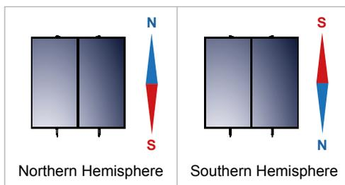
**Orientation - optimum angle:** a basic factor for the system's optimum performance is the selection of its angle and orientation for its particular location and the time during which the maximum gain is required. The solar system should be positioned so that the collector's surface faces the geographical south, if the installation takes place in the Northern Hemisphere (and the geographical north for the Southern Hemisphere), i.e. it should always face the Equator.
