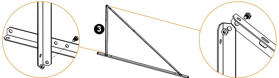
3. Screw diagonal part 4 to the above parts and tighten all screws. Repeat steps 1, 2 & 3 for the other pairs of parts.
