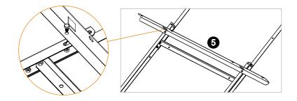
5. Bend the straight parts **6** of step 2 with the hand covering the beams of the tiled roof. Drill and fasten up with bolts. Use level so that the base is horizontally placed.
