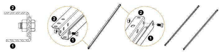
Place part 4 between the two Π shape parts constructed in the former step 1 in order for the frame to be formed. Screw straight parts 6 (which will be used for the mounting of the support base to the tiles) to the botton part. Repeat for the rest of the parts.
