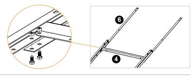
Screw the collector supporting part 5 to the bottom part of the frame and tighten the screws.
