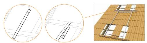
6. In case of two collectors, first place the left one at the bottom part **5**, lifting the upper part **5**. Place the screws and the collector's fixing washers (4 for each collector) without tightening them. Place mechanically tightened Ø22 unions at the edges of the collector.
