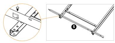
Screw the collector supporting part 5 to the top part of the frame without tightening the screws.
